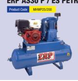
British built and powered by a 11hp petrol electric start engine. 150lt receiver and 150psi max pressure, supplied with rubber mounts as standard. A real workhorse.
