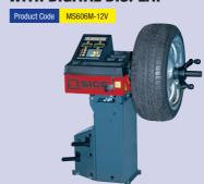
Conceived for mobile wheel service units or usage where space is limited, this extremely easy to use hand spin machine needs just a 12volt supply to operate. Manual brake and 11 balancing programmes for steel and alloy passenger car, van and motorcycle wheels. Complete with special OPT and Hidden Weight programmes.
